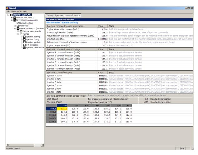
The map of target of injectors command tension allows to choose the tension with which injectors must be piloted, between 115 volts and 180 volts.
