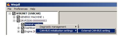
The CAN-bus speed is fixed to 1 Mbits.
