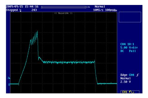
In this try, the current increases: the passive times are too short and the active times too long. After some tries, the withstand of the current is obtained.
