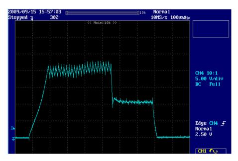
during the reiterations, the current goes back up a little: a last retouch is necessary: the passive time of the couple #8 (the one which is repeated) will be slightly increased from 12 to 13, and the desired result is obtained (oscillogramme presented at the beginning of chapter).
