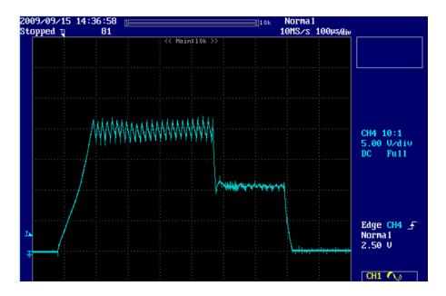
We distinguish the attack there during which the current quickly goes up in some dozens of microseconds, and a first level of switching regulation, the withstand.
