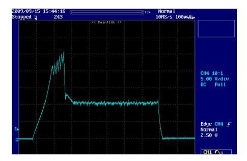
In this try, the current increases: the passive times are too short and the active times too long. After some tries, the withstand of the current is obtained.
